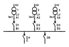
E.g. If transformers 1, 2 & 3 were rated at 630kVA each, circuit breakers D1, D2 & D3 must have a breaking capacity u 42kA.
